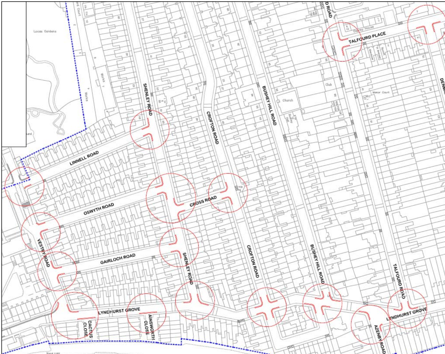
Figure 15 – Proposed no waiting at any time (double yellow lines) on junctions
